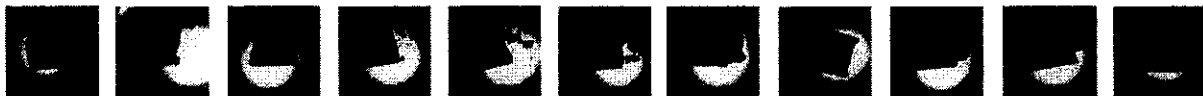
Figure 5. Photographs of a sequence of deuterium pellets from TPOP-II injector (8-mm bore); pellets fired at 0.5 Hz and \sim 1 \text{ km/s} .
